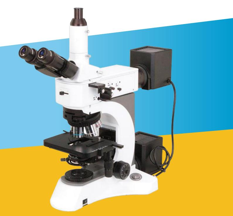
Upright Metallurgical microscopes LD-LMM-B11 and LD-LMM-B12 with siedentopf trinocular head design, infinite optical system, reflected & transmitted Kohler illumination system meets performance demands of metal, plastic, electrical circuits & engineering industry. Its superior coaxial course and fine focusing tension adjustment knobs helps in better examination of samples.
