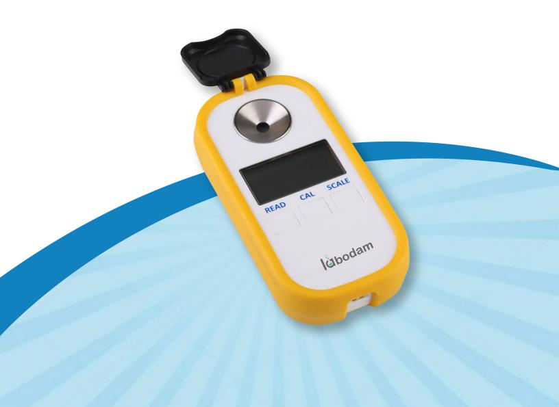
Portable brix refractometer is a microprocessor controlled pocket sized optical instrument that provides instant measurement readings. Automatic temperature compensation (ATC) eliminates temperature corrections between 0 °C to 40 °C. Automatic power off post one minute of last operation prolongs it's battery life. Ideal for determining brix concentration of fruits, beverages, oils and organic solvents.
