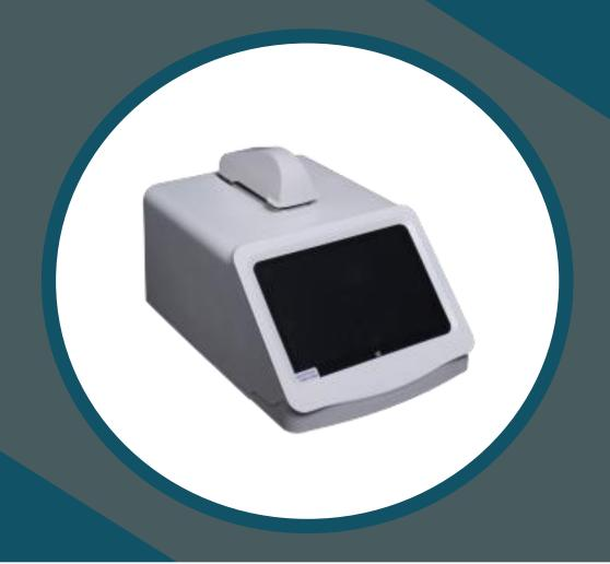
Nano Spectrophotometer LD-LNS-A30 is a benchtop unit comprises wide wavelength range of 190 to 850 nm, 0.3 - 2  $\mu$ l micro volume sample measurement, and 1 mm, 0.05 mm, optical path length. With built-in detection system, and high definition, touch screen display it offers less than 5 seconds of detection time. Easy to transfer test Data via USB port or Network. Incorporated with Xenon flash lamp as light source with high stability and long operating life.
