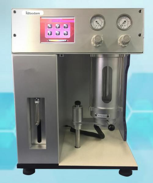
Liquid Particle Counter LLPC-A10 comes with high precision syringe sampling and semiconductor laser sensor. Designed using photoresist method principle, it detects size and number of solid particles in a liquid sample. It's a high quality performance instrument, designed in accordance with international standards such as ISO4406:1999.
