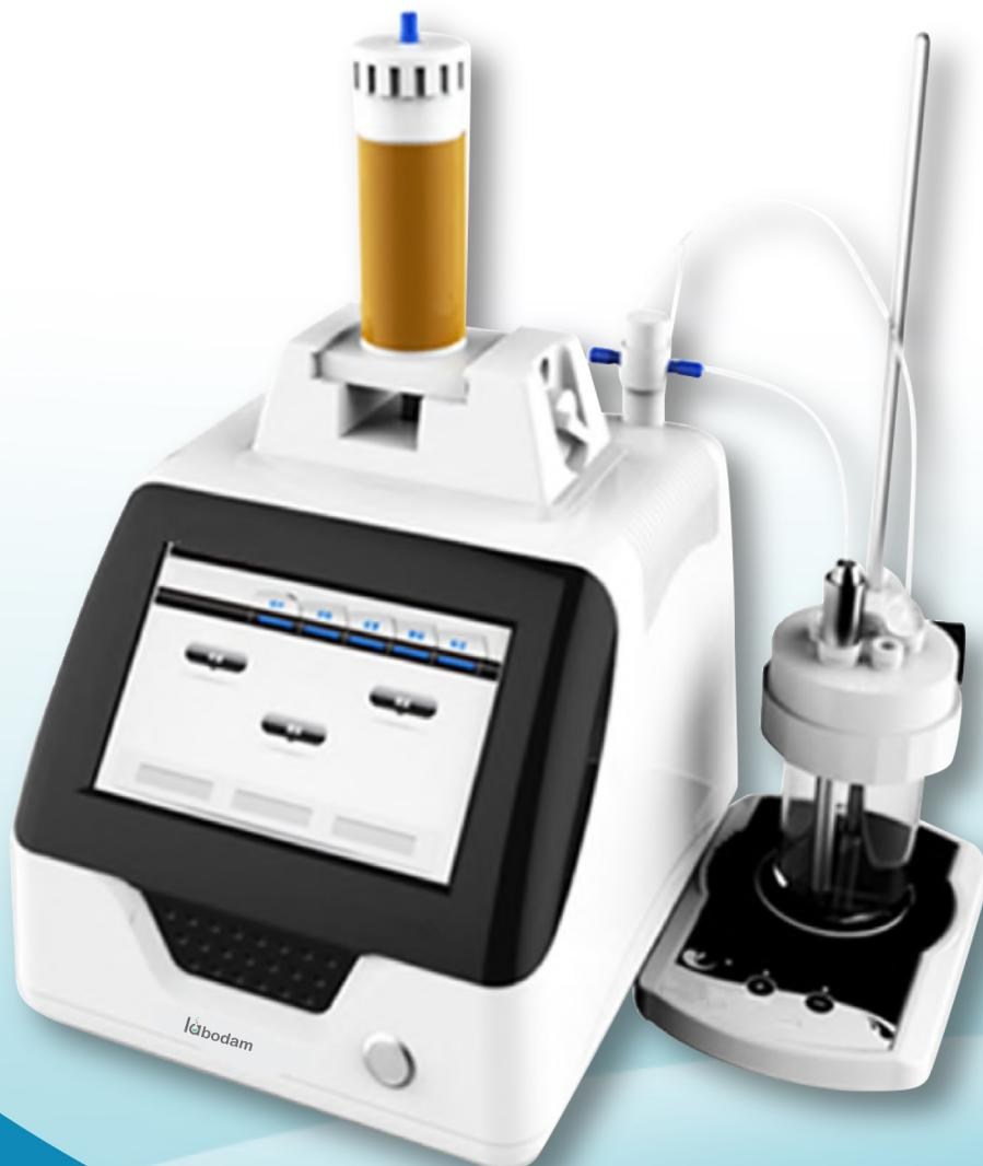
Automatic Potentiometric Titrator LPTT-A10 is an automatic titrator with integrated burette valve design. This modular titrator consist of three units: volume titration device, control device, measurement device. The titration analysis includes acid-base titration, oxidation-reduction titration, non-aqueous, precipitation titration and others.
